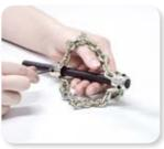
1 Loosen the screws on both sockets on the chain. Bring the shaft / cable through both sockets.
